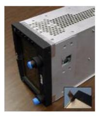
34. \_\_\_\_Carefully Peel back aluminum tape from the bottom of the unit (the tape is to be reapplied at the end of this procedure). Leave attached to the cover.
