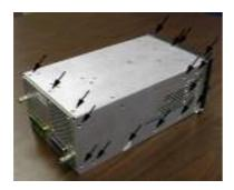
35. \_\_\_\_\_Remove the 24x #4-40 Flathead Screws, and 3x black #4-40 Flathead Screws.
