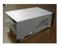
37. \_\_\_\_\_Slide cover back – front end may "stick" for first half-inch of travel.
