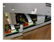
47. \_\_\_\_\_Insert white Flex-Cable into ZIF connector. Make certain it is inserted until the cable hits the stop. Push top of ZIF connector down.
