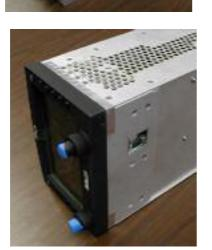
49. \_\_\_\_\_Re-assemble cover with 24x #4-40 Flathead Screws and 3x black #4-40 Flathead Screws.
