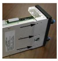
45. \_\_\_\_\_Re-assemble Display Assembly with 3x #4-40 Flathead Screws.
