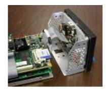
43. \_\_\_\_Slide Display Assembly forward.
