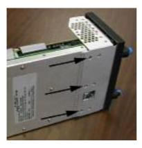
42. \_\_\_\_Remove the 3x #4-40 Flathead Screws from bottom of Display Assembly cable which connects the cover to the chassis.
